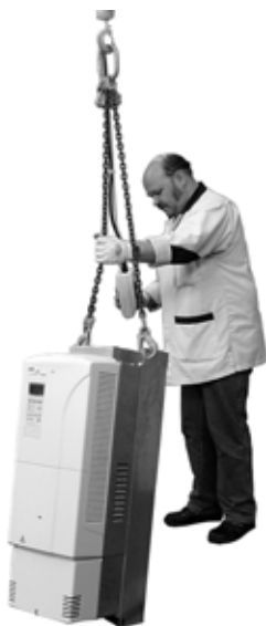
Lifting a unit of frame size R6
