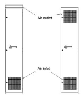
Arrange the cooling of the modules so that the requirements given in chapter *Technical data* are met:
