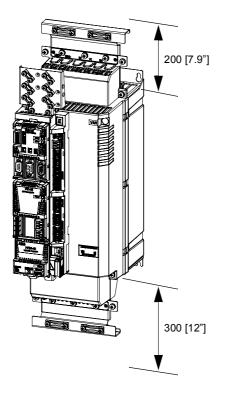
The temperature of the cooling air entering the unit must not exceed the maximum allowed ambient temperature (see *Ambient conditions* in the chapter *Technical data*). Consider this when installing heat-generating components (such as other drives, mains chokes and braking resistors) nearby.
