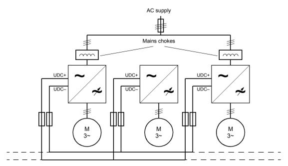
Each drive has an independent DC capacitor pre-charging circuit.
