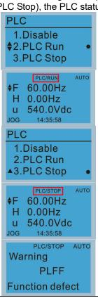
Choose option 2: PLC Run to enable the PLC function.
