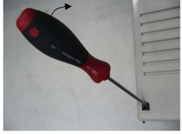
Remove the DCS Control Panel, if present. Depress the locks to remove the cover
