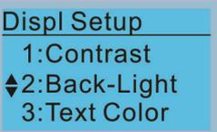
When the setting value is 10 Min, the backlight turns off in 10 minutes.
