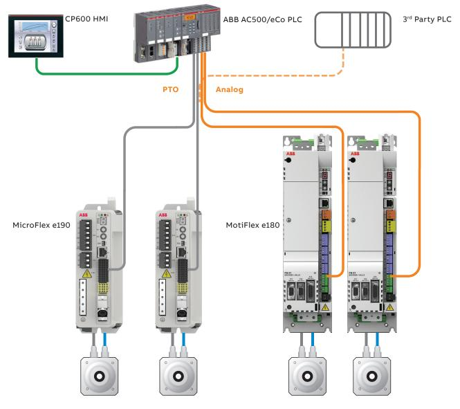
Rotary/linear servo motors
