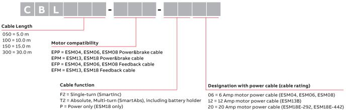
20 = 20 Amp motor power cable (ESM18E-292, ESM18E-442) 35 = 35 Amp motor power cable (ESM18E-552, ESM18E-752) 2 = Feedback cable with 15 way D Type fitted
