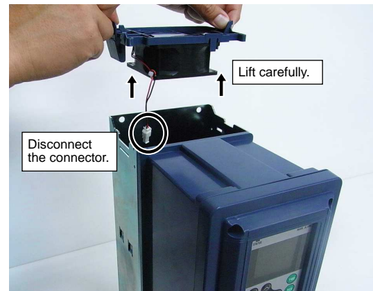
Remove cooling fan cable (connector). Remove and replace the fan case and cooling fan.
