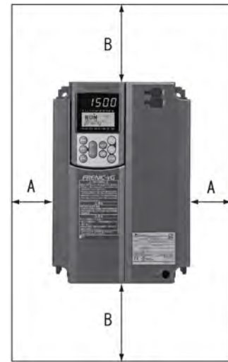
Figure 3.3-1 Mounting Direction and Required Clearances
