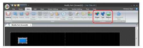
3. When editing other patterns of the switch, click [View] → [State Change] to select a pattern from [OFF], [ON], [P3] and after, and then edit according to step 2.
