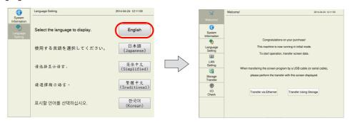
Press [Transfer via Ethernet] or [Transfer Using Storage] to switch the screen.
