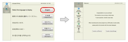
2. Press the [Transfer via Ethernet] switch to display the [LAN Setting] screen.
