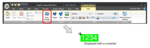
2. The item view window for the placed data display is displayed on the screen. (If the view window does not appear, double-click the data display.)
