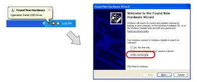
3. Select [Install the software automatically] on the [Found New Hardware Wizerd]. Click [Next] to install the USB driver.
