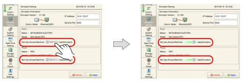
When running the simulator for PLC 1 and PLC 2, for example, set the switch for both of these to [Use (Simulator)].
