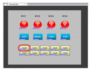
1. Double-click the "D100" field on the simulator. The [Write Device] window is displayed.
