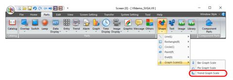
2. Drag the mouse from the start point to the end point in the same way as drawing a rectangle. The trend graph scale is drawn.
