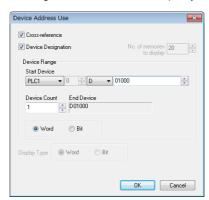
3. Click [OK] to display a tab window that shows the usage status of device memory addresses in the specified range.
