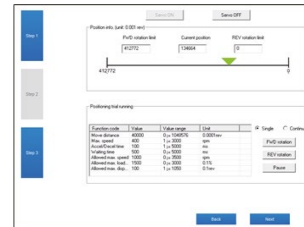
Easy auto-tuning using position JOG and self-adjustment
