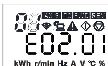
Figure 3-4 Fault code displayed on the operating panel
