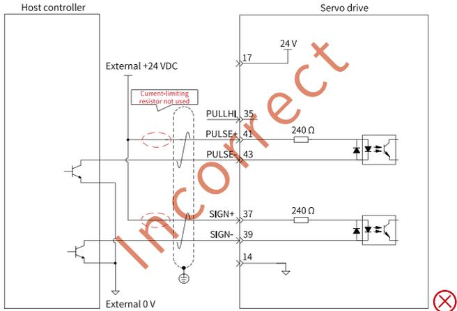
Figure 4-8 Incorrect wiring example 1: The current limiting resistor is not connected, resulting in terminal burnout.
