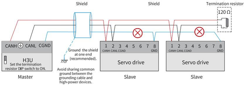
Figure 3-11 Incorrect CAN connection way
