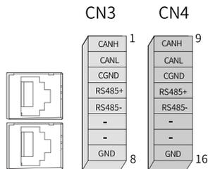
Figure 4-18 Communication Terminal pin layout of the servo drive
