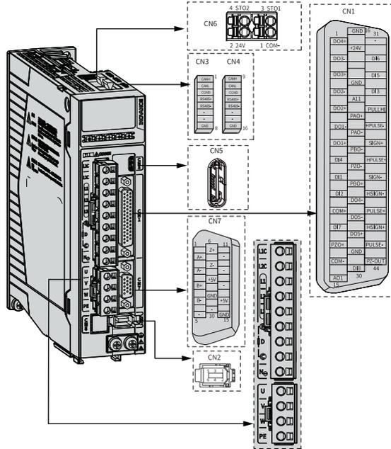
Figure 4-1 Terminal pin layout of the servo drive
