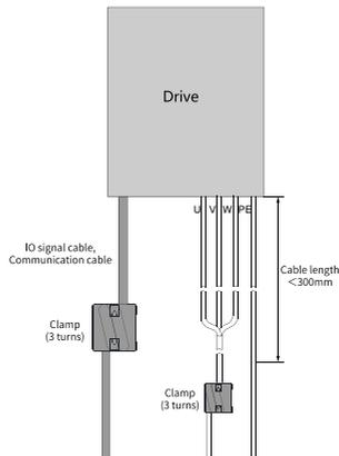
Figure 3-4 Connection of the magnetic buckle
