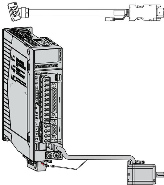
Figure 4-16 Wiring example of absolute encoder signals<sup>[1]</sup>
