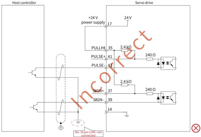
Figure 4-7 Incorrect: Pin 14 (COM-) is not connected, leading to failure in forming a closed-loop circuit.
