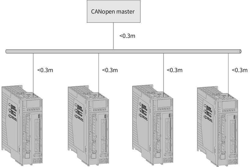
Figure 3-13 CAN communication network topology
