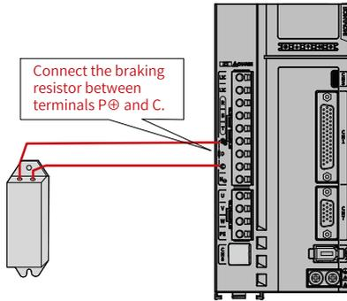
Figure 3-5 Wiring of external regenerative resistor
