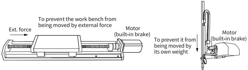
Figure 4-13 Application of the brake
