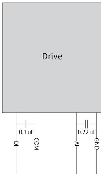
Figure 6-2 I/O signal cables with capacitance increased
