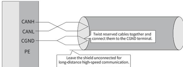
Figure 3-19 Recommended connection mode 5
