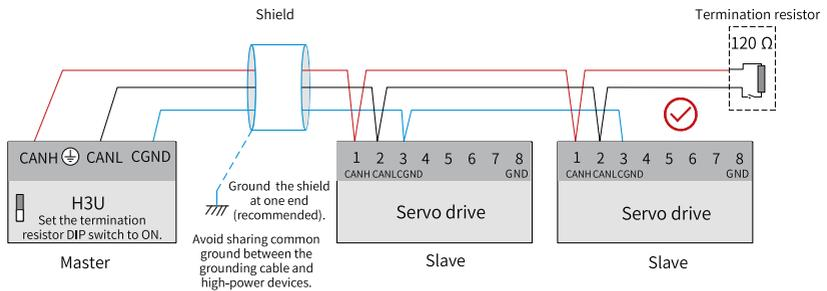
Figure 3-10 Correct CAN connection way
