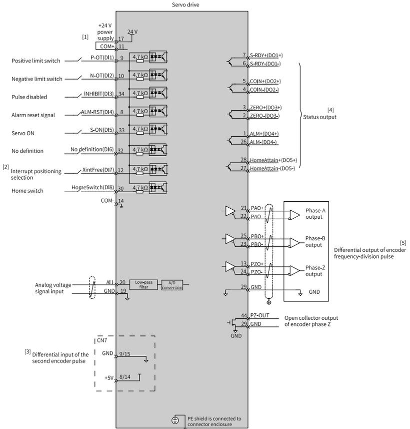
Figure 2-2 Wiring Diagram for Torque Control Mode
