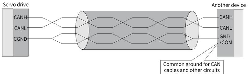
Figure 3-20 Connection mode for sharing the ground with other circuits
