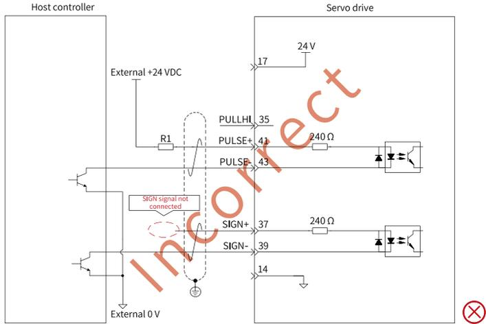
Figure 4-10 Incorrect wiring example 3: The SIGN port is not connected, preventing these two ports from receiving pulses.
