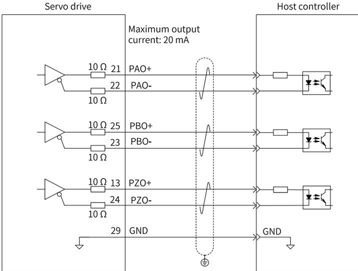
The encoder phase Z frequency-division output circuit supports open-collector signal output. Typically, this circuit provides feedback signals to the host controller in a position control system. Use an optocoupler circuit, relay circuit, or bus receiver circuit on the host controller side to receive feedback signals.
