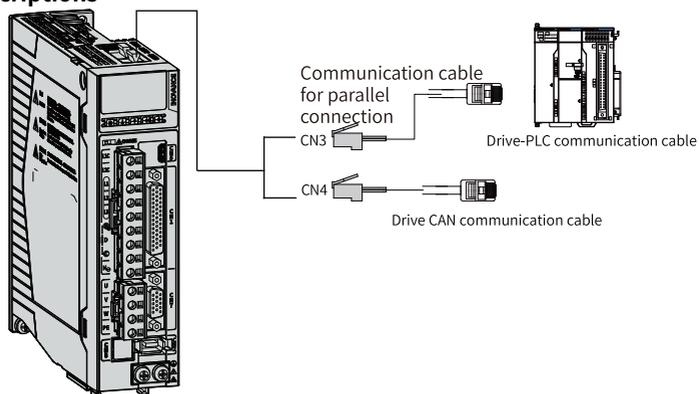
Figure 4-19 Wiring of communication cables
