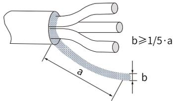
Figure 3-8 Lead-out of the motor cable shield
