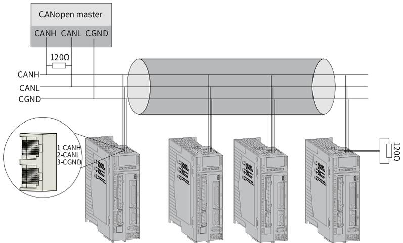
Figure 3-14 CANopen wiring diagram
