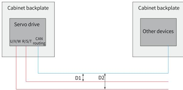
Figure 3-22 Recommended routing modes
