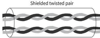
Figure 3-9 Diagram of shielded twisted pairs
