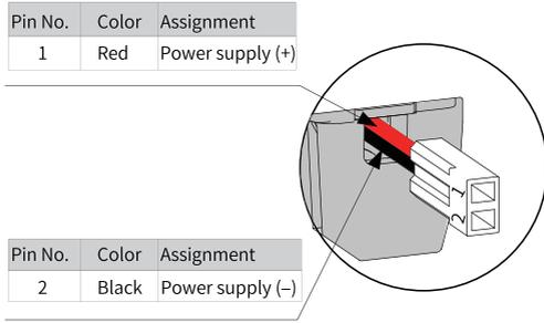
Figure 4-17 Description of the lead wire color of the battery box
