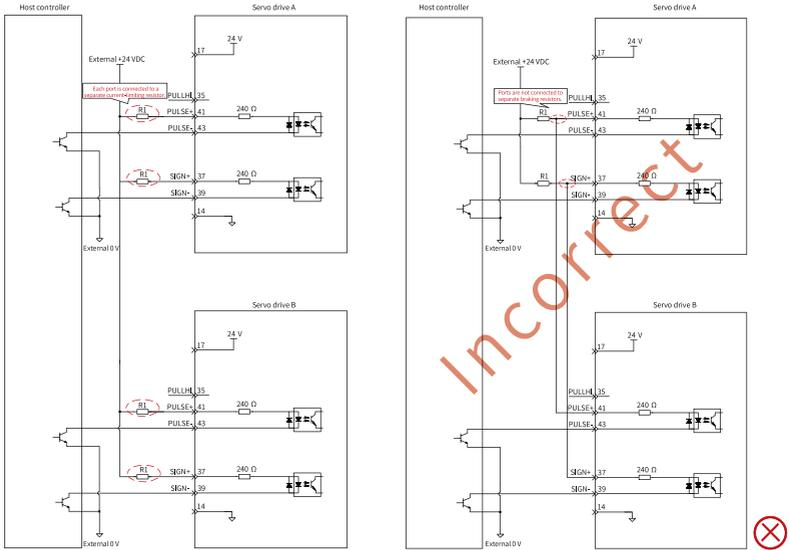
Figure 4-12 Incorrect wiring example 5: Multiple terminals share one current limiting resistor, resulting in a pulse receiving error.
