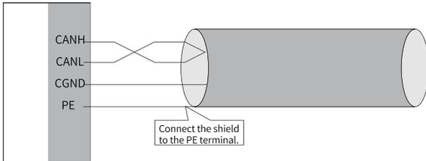
Figure 3-16 Recommended connection mode 2
