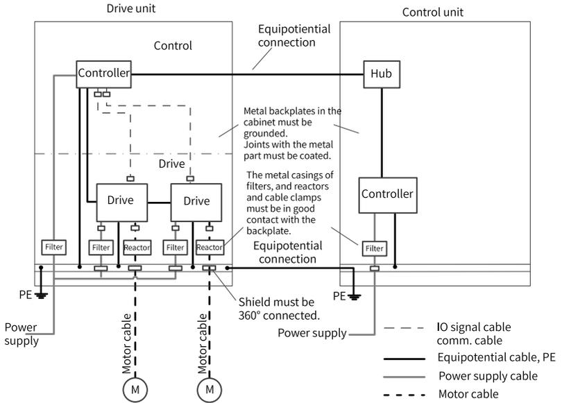
Figure 3-28 Recommended wiring for the control cabinet system
