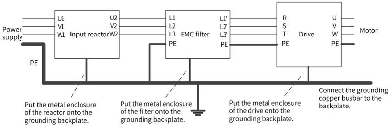
Figure 3-1 Connection of the AC input reactor
