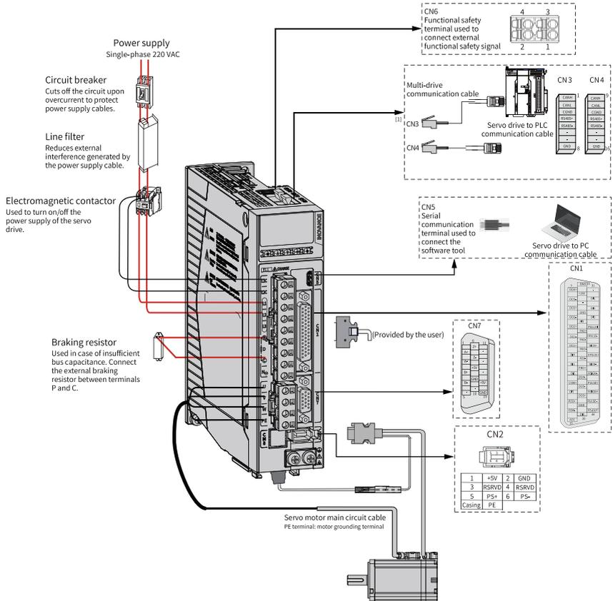
Figure 1-1 Example wiring of a single-phase 220 V system
