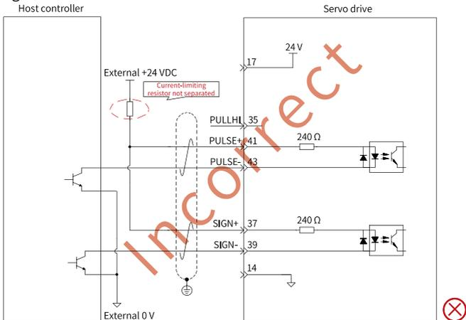
Figure 4-9 Incorrect wiring example 2: Multiple terminals share the same current limiting resistor, resulting in pulse receiving error.
