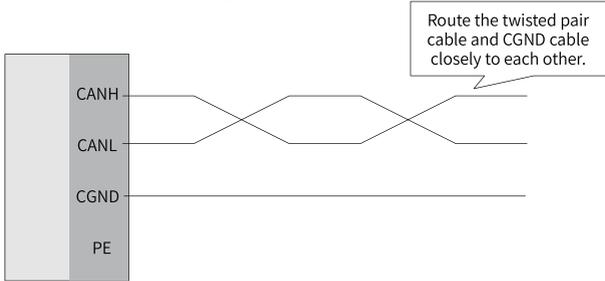
Figure 3-15 Recommended connection mode 1
