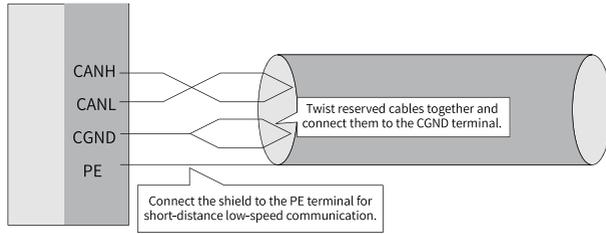
Figure 3-18 Recommended connection mode 4
