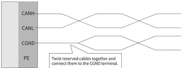
Figure 3-17 Recommended connection mode 3
