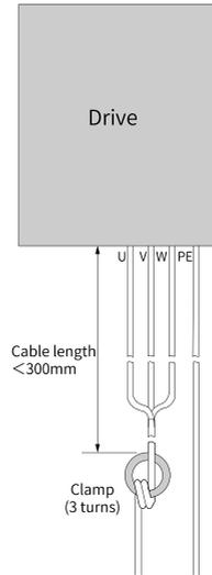
Figure 3-3 Connection of the magnetic ring
