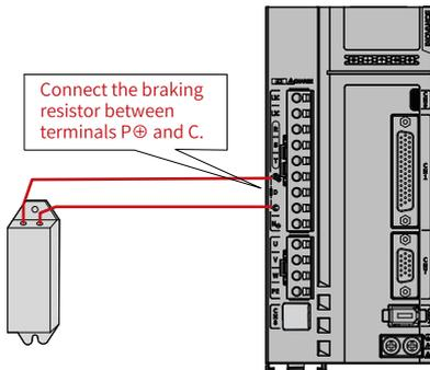
Figure 4-24 Wiring of external regenerative resistor
