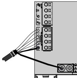
Figure 3-7 Connection of the shielding layer
