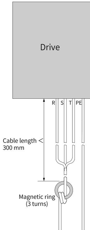
Figure 6-1 Magnetic ring on the input side
