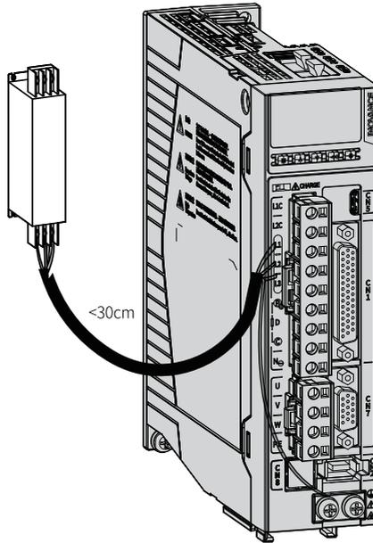
Figure 3-2 Connection of the EMC filter
