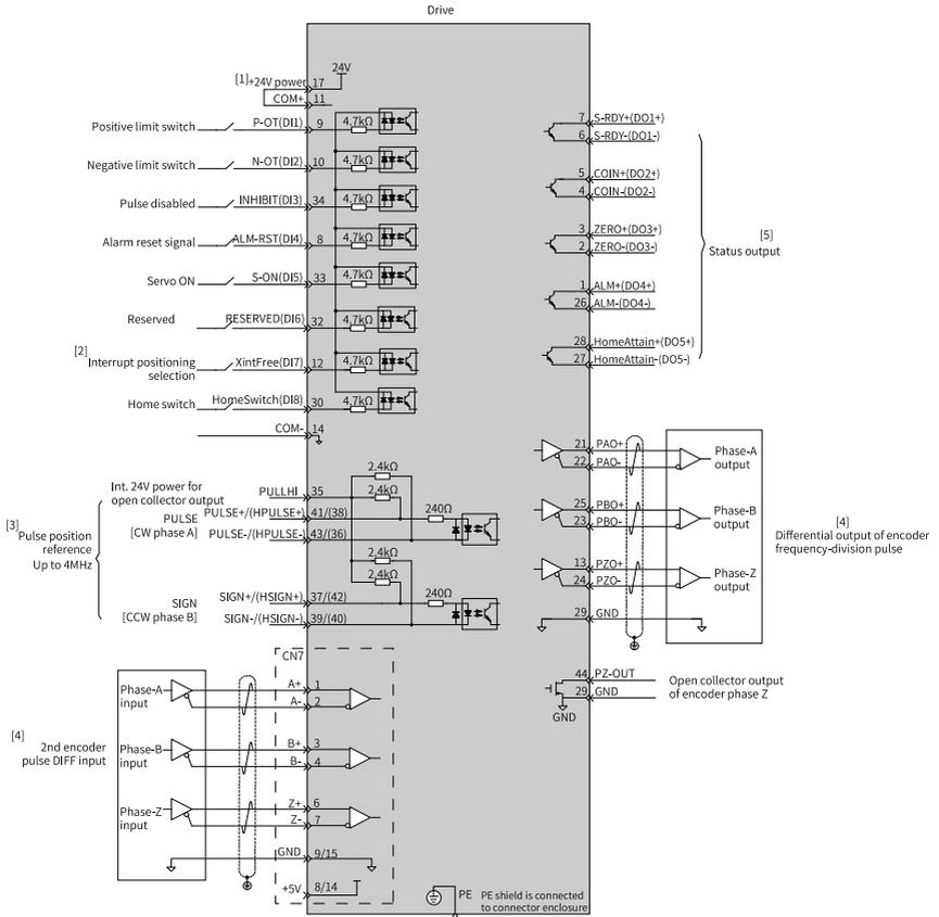
Figure 2-1 Wiring diagram of the Position Control Mode
