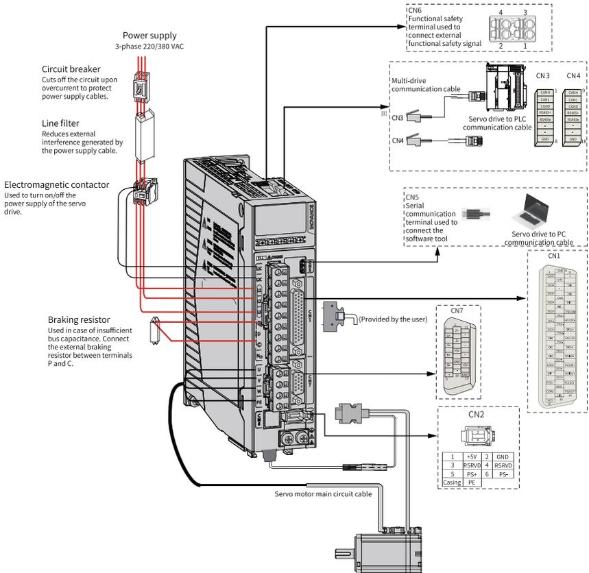
Figure 1-2 Example wiring of a three-phase 220 V or 380 V system
