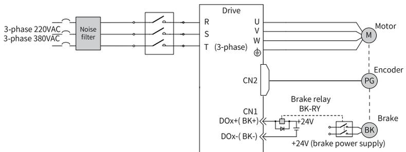
Figure 4-14 Wiring of the brake
