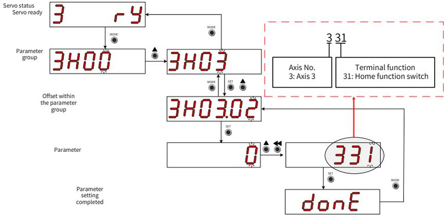
Figure 4-8 Procedures for DI function setting
