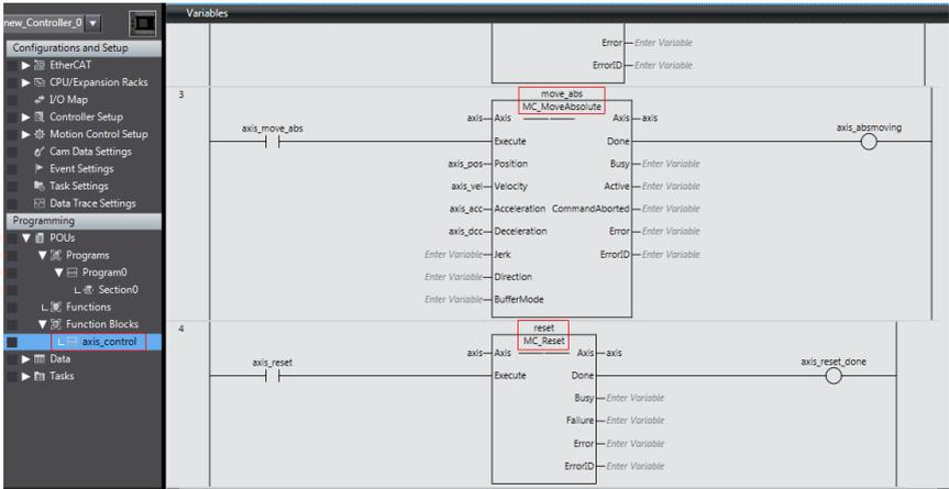
Call the function block in section0, and you can make the shaft rotate through the bus.
