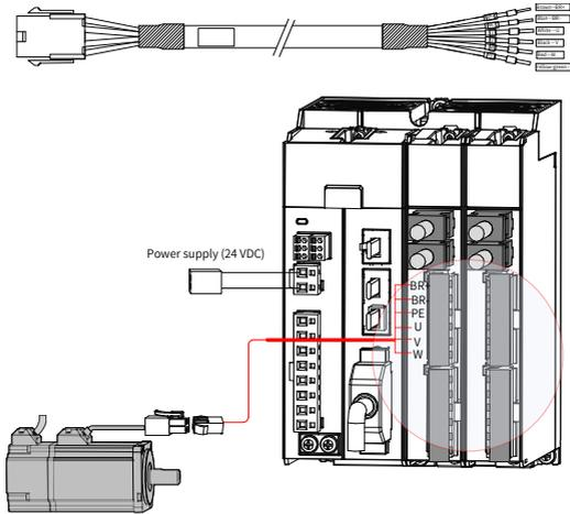
Figure 3-7 Example of the wiring between the servo drive and the motor with brake
