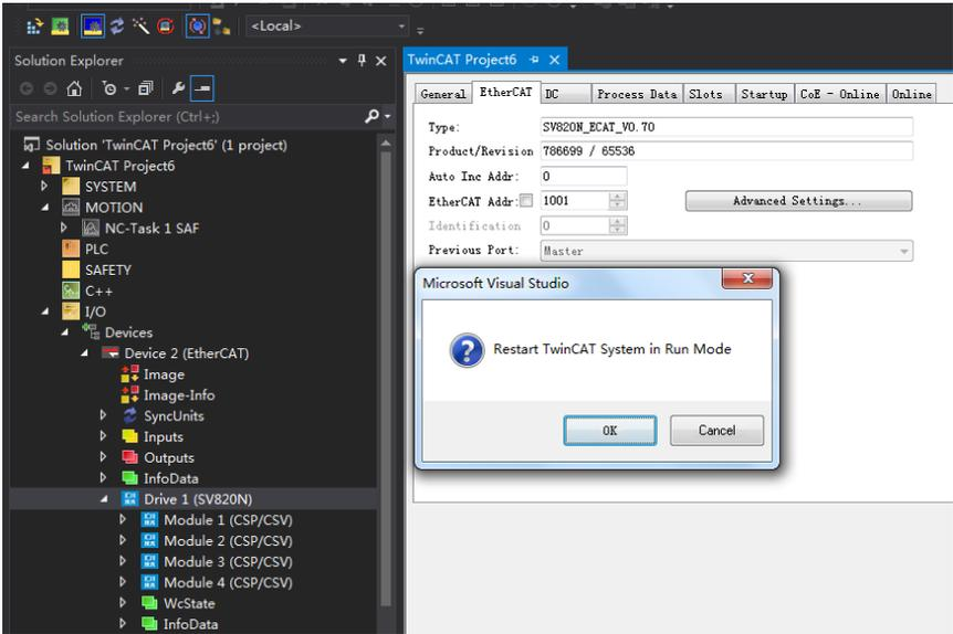
After clicking **OK**, you can observe through the **Online** interface that the device enters OP status, and the second LED on the servo drive keypad displays "8", and the keypad displays "1\_88RY".
