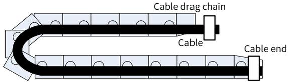
Figure 3-23 Cable drag chain
