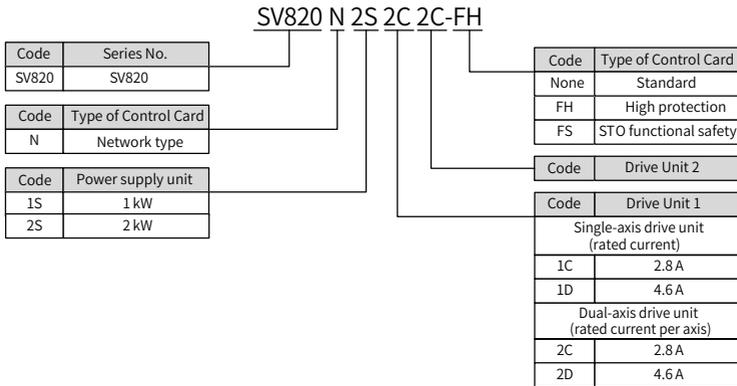
Note: Motors of 400 W (inclusive) are configured with 2C or 1C drive unit.
