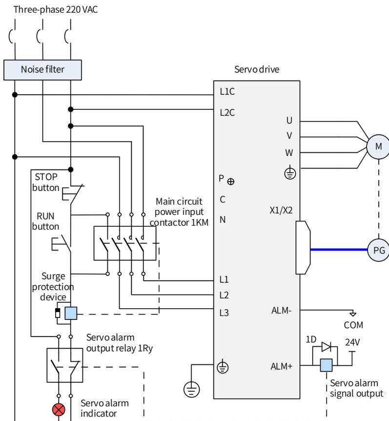
Figure 3-6 Main circuit wiring of three-phase 220 V models
