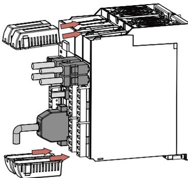
Figure 3-13 Installation of the absolute encoder battery box
