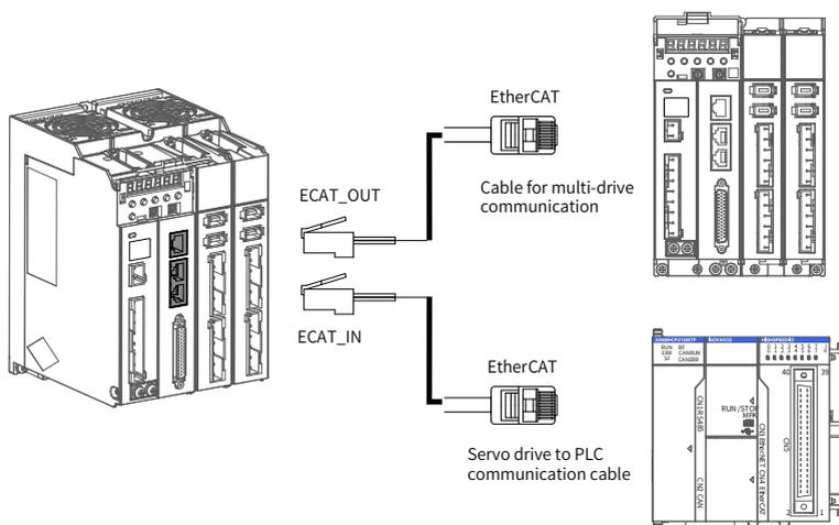
Figure 3-16 Wiring of communication signals
