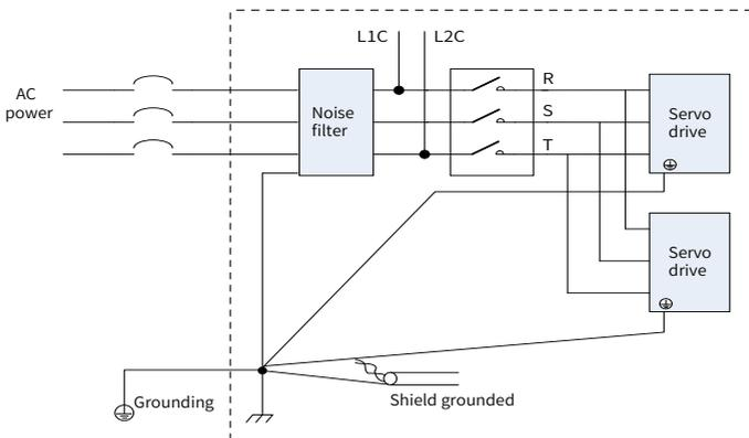
Figure 3-22 Grounding of the noise filter
