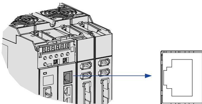
Figure 3-17 Ethernet connector terminal
