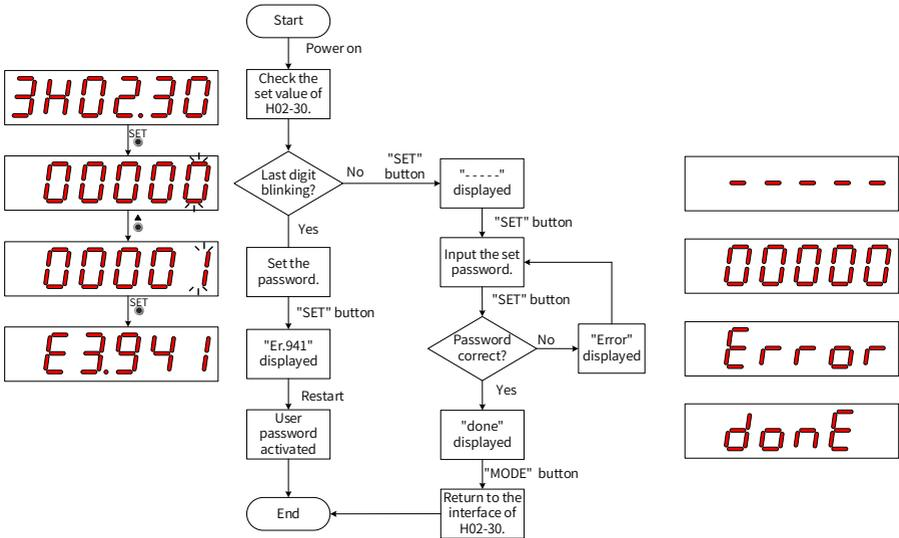
Figure 4-6 Procedures for user password setting
