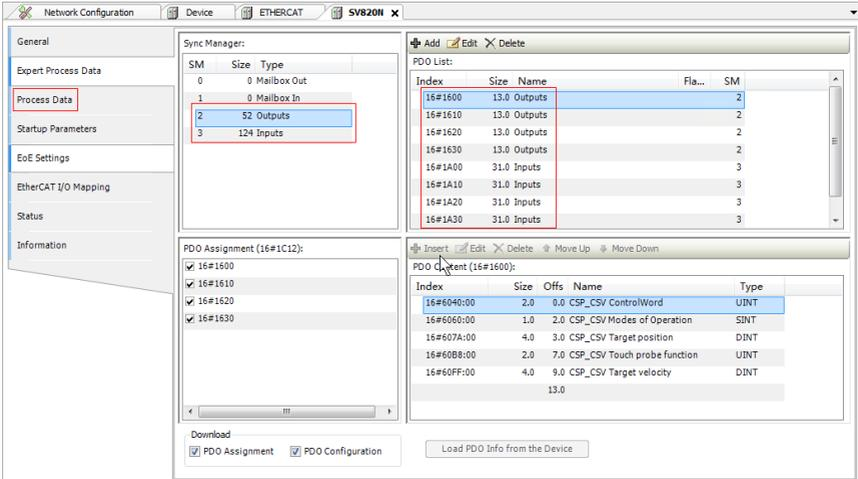
The PDO list configured according to the CSP (Position) + CSV (Velocity) + TP (Touch Probe) mode is as follows.
