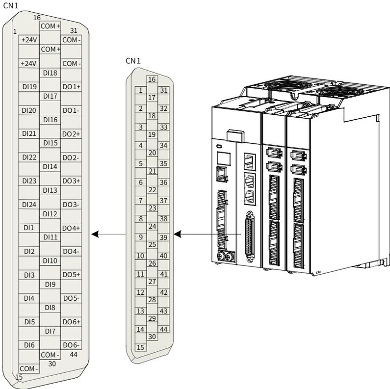
Figure 3-14 Pin layout of control circuit terminal connector
