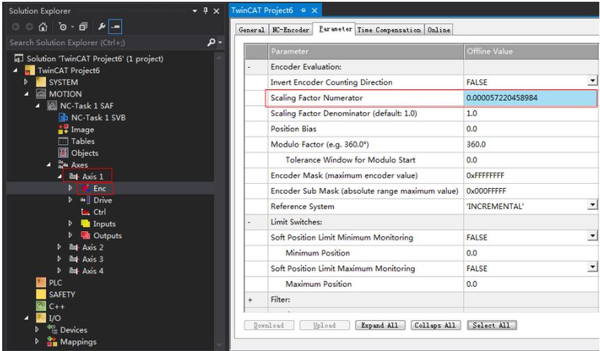
Click **Axis 1** in **Axes**, select **Parameter**, and hide the system deviation temporarily (same as other axes).
