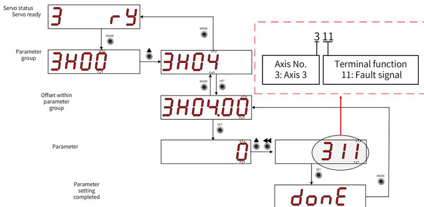
Figure 4-9 Procedures for DO function setting
