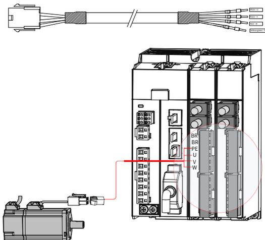
Figure 3-8 Example of the wiring between the servo drive and the motor without brake
