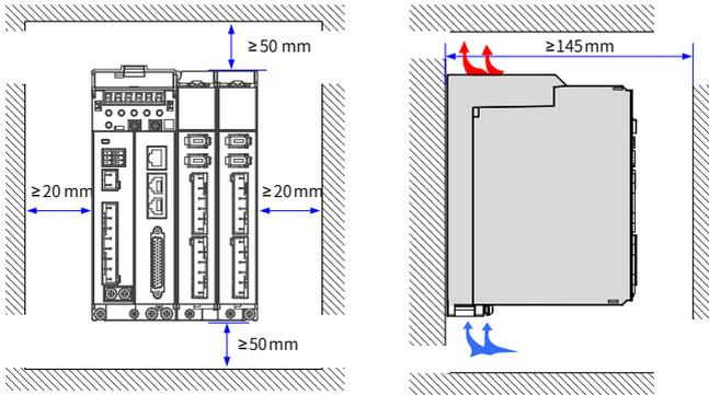
Figure 2-4 Installation clearance
