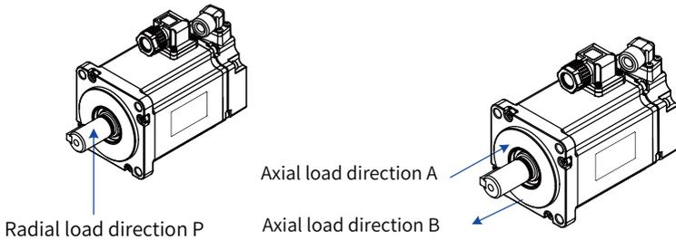
Figure 1-8 Radial and axial loads of the motor
