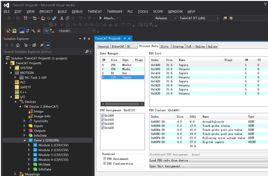
The screenshot shows the TwinCAT Project6 configuration interface in Microsoft Visual Studio. The left pane displays the Solution Explorer with the project structure, including the 'Devices' folder and 'Device 2 (EtherCAT)'. The right pane shows the 'EtherCAT' configuration tab, which includes a 'Sync Manager' table, a 'PDO List' table, and a 'PDO Content' table.
