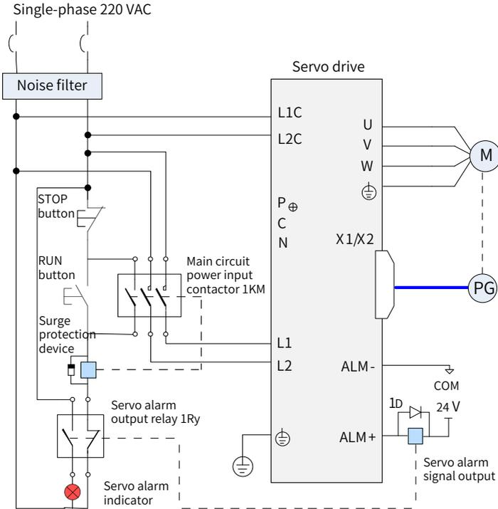
Figure 3-5 Wiring of the main circuit of single-phase 220 V models
