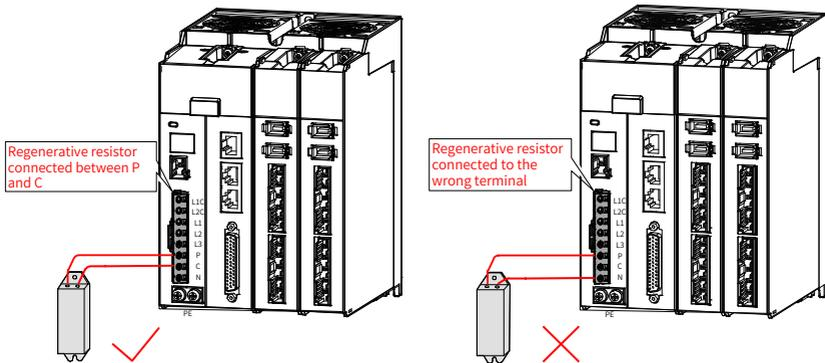
Figure 3-3 Connection of the external regenerative resistor
