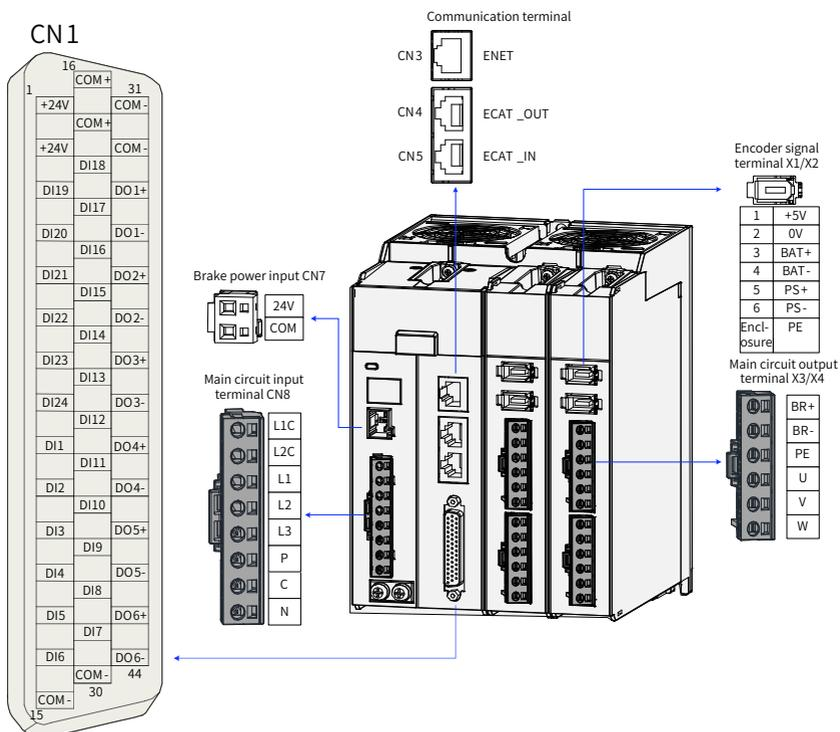
Figure 3-1 Terminal pin layout
