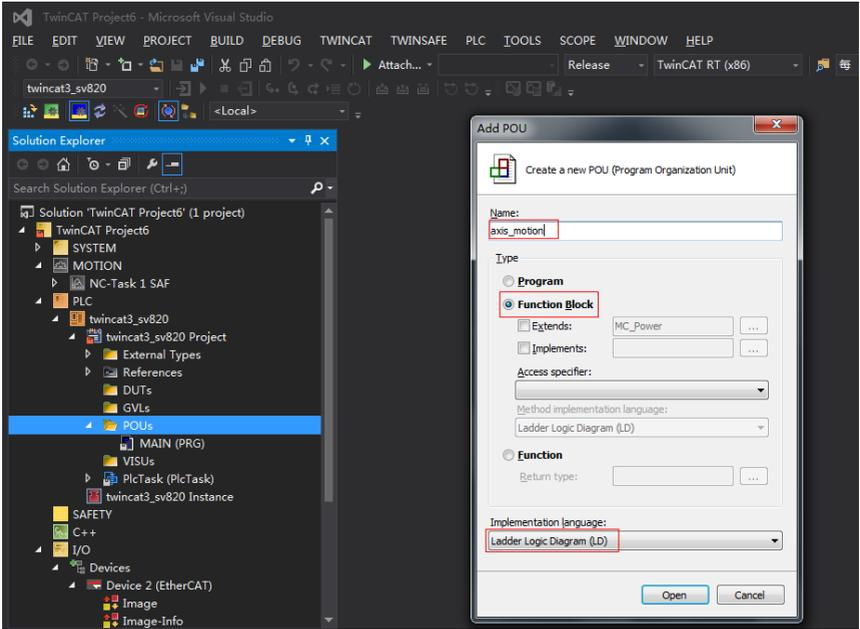
Create a new FB and add **MC\_power**, **MC\_jog**, **MC\_home**, **MC\_absolute** and **MC\_reset** to FB.
