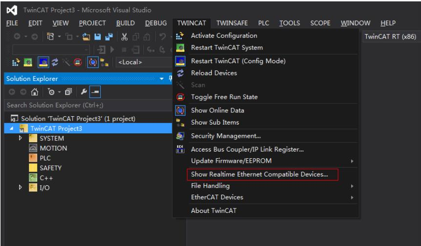
Open **Show Realtime Ethernet Compatible Devices...** in the menu shown in the preceding figure. In the pop-up dialog box shown below, select local network in **Incompatible devices**, and click **Install**. After the installation is done, the network card installed is displayed in **Installed and ready to use devices**.
