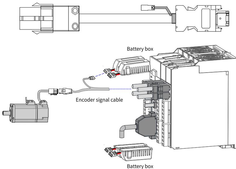
Figure 3-11 Wiring example of absolute encoder signals and the battery box
