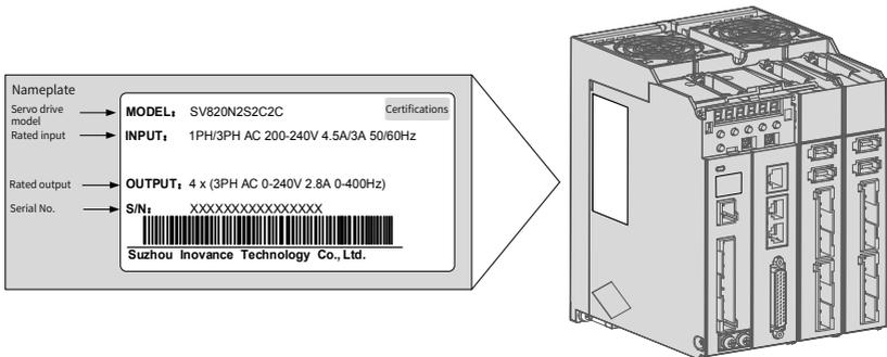
Figure 1-4 Description of the servo drive nameplate
