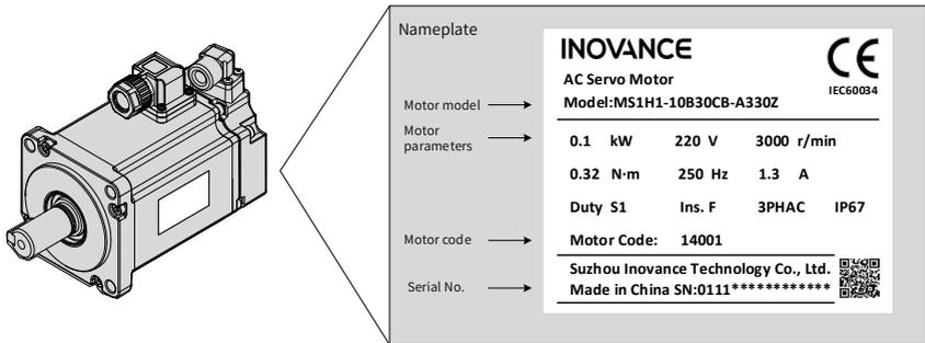
Figure 1-6 Description of the servo motor nameplate
