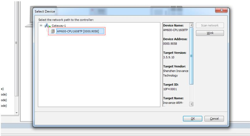
Select the AM600 device scanned. Now the communication connection between PLC and PC is established. Next, configure the device.
