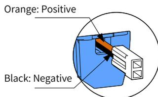
Figure 3-12 Description of the lead wire color of the battery box
