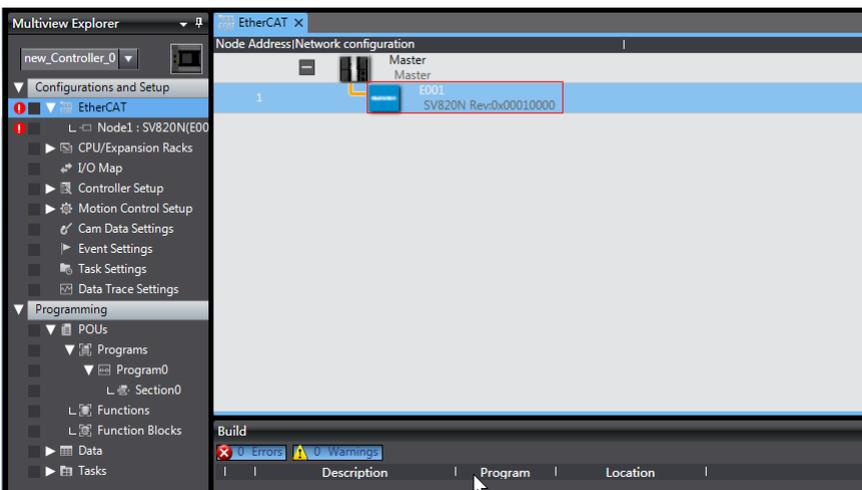
The SV820N is a 4-in-1 servo drive with PDO list pre-planned for easy use of each axis. Select a mode you need from "CSP/CSV+TP, CSP+TP, CST, CSP/CST+TP, CSP/CST/CSV+TP, PP+TP, PP\PV\PT+TP", and the PDO list needed by this mode will be selected by XML files through working with the controller. All the axes in this application example are selected with CSP/CST/CSV+TP mode.
