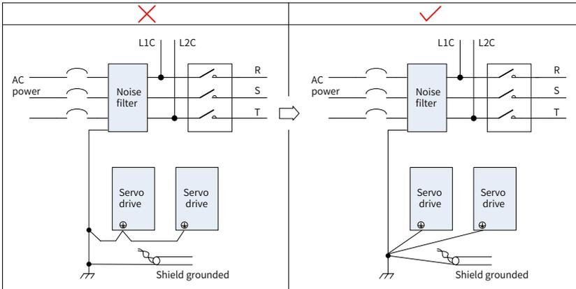
Figure 3-21 Single-point grounding
