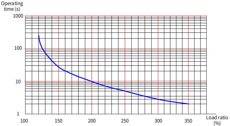
Figure 1-7 Motor overload curve
