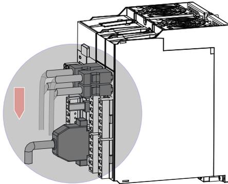
Figure 2-6 Routing direction
