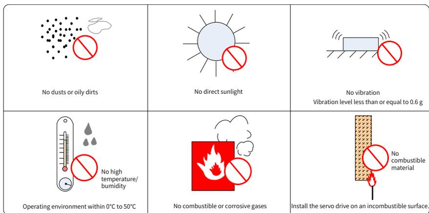
Figure 2-1 Installation Environment
