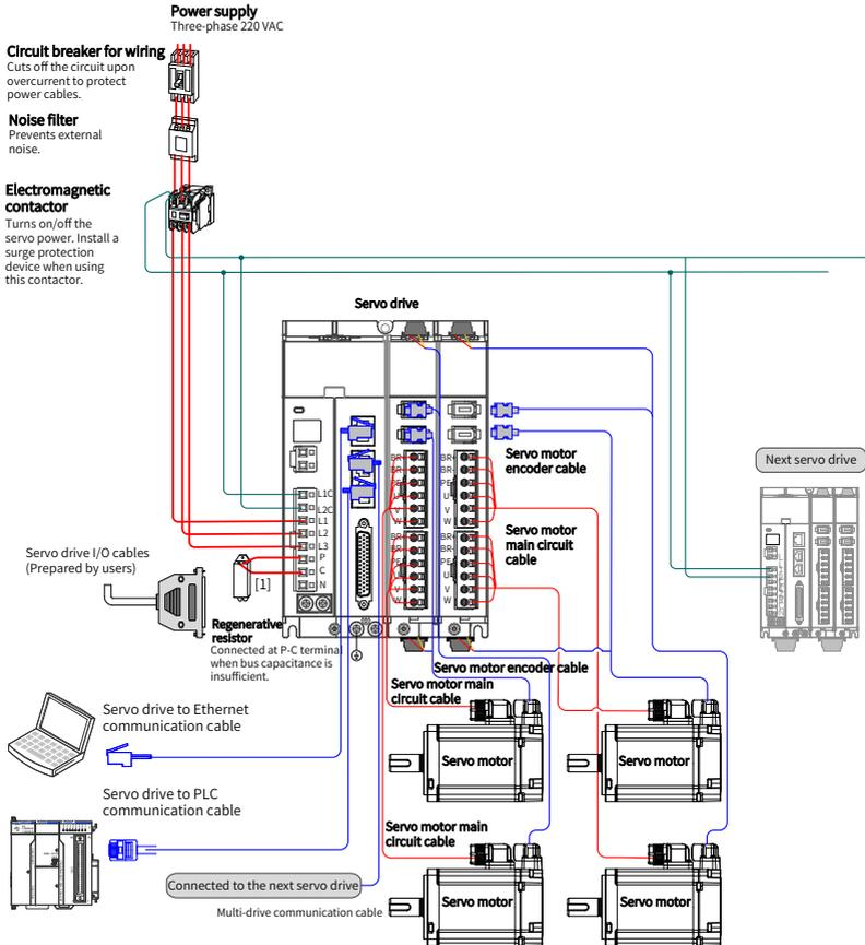
Figure 1-2 Wiring example of the three-phase 220 V system
