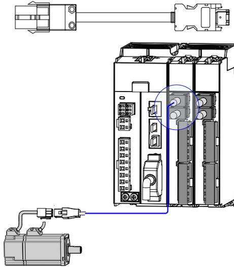
Figure 3-9 Wiring example of encoder signals
