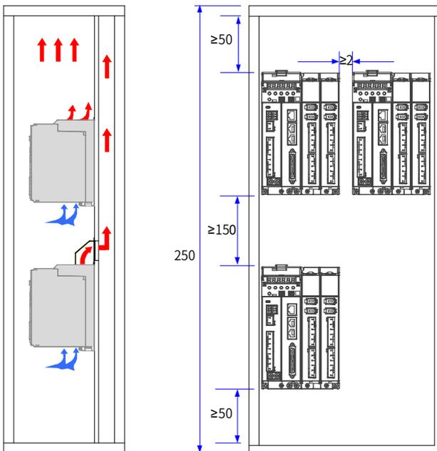
Figure 2-3 Dual-row installation clearance
