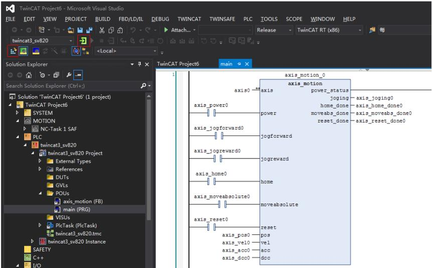
Click the arrow indicated by the red box to start the PLC. After the PLC starts running, you can run the servo drive through the bus.
