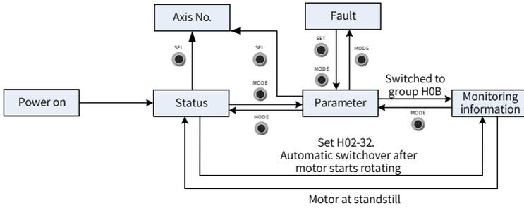
Figure 4-2 Switchover between different types of display
