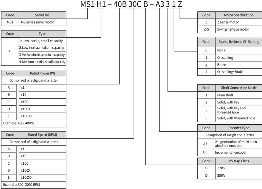
Figure 1-5 Description of the servo motor model number
