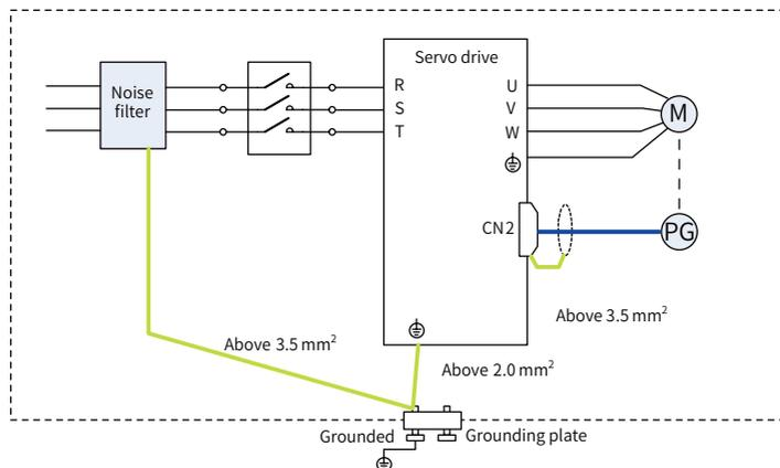
Figure 3-18 Anti-interference wiring example
