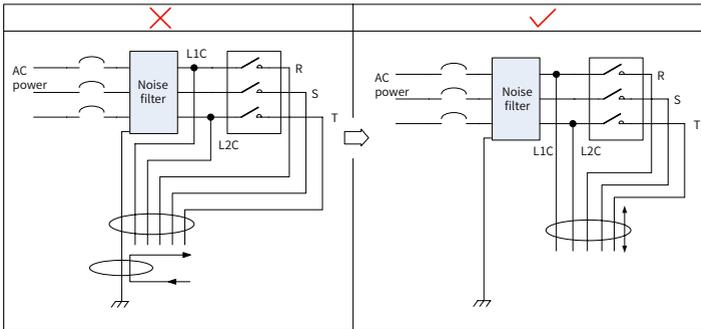
Figure 3-20 Separate routing of the grounding cable and output cable
