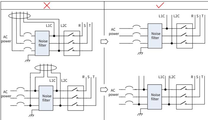
Figure 3-19 Separate routing of I/O cables of the noise filter
