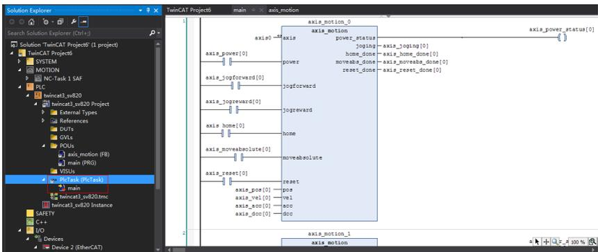
Compile the program. If there is no fault, configuration can be activated, and then log onto the PLC.
