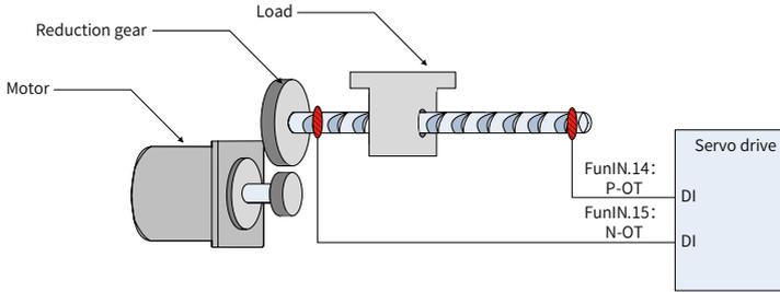
Figure 6-1 Installation of limit switches
