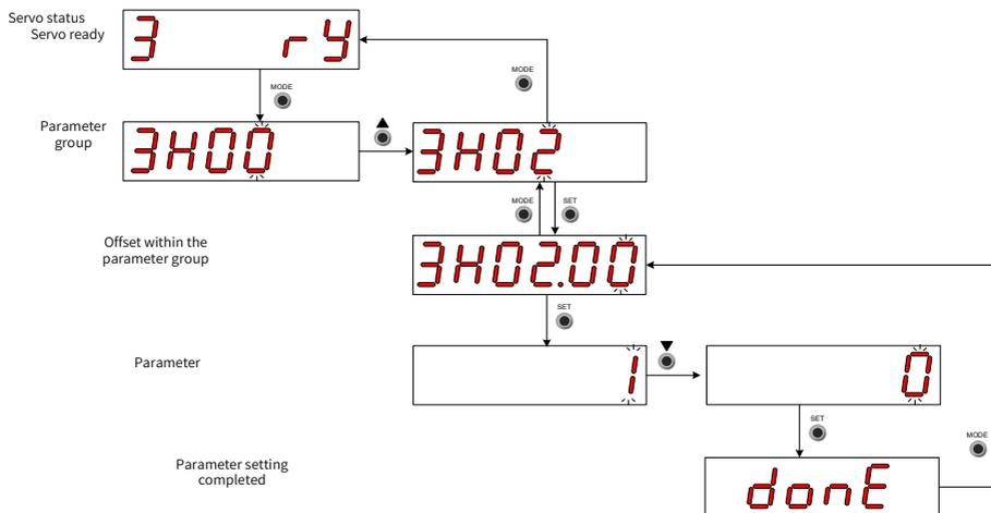
Figure 4-5 Procedures for parameter setting
