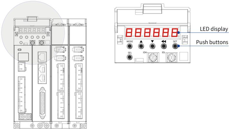
Figure 4-1 Appearance of the keypad
