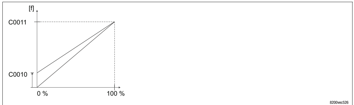
Fig. 7-5 Relation between setpoint and minimum and maximum output frequency
