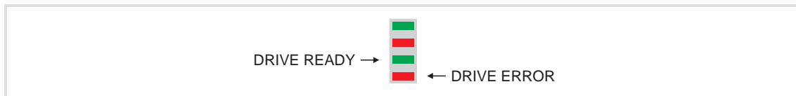
[10-2] DRIVE READY and DRIVE ERROR LED status displays
