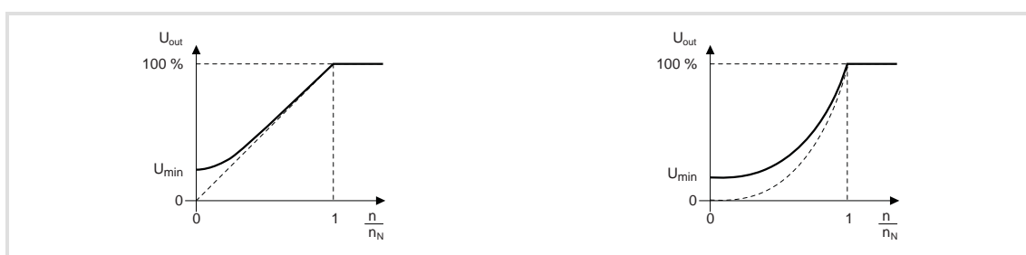
[5-3] Principle of a linear V/f characteristic (on the left) and a quadratic V/f characteristic (on the right)
