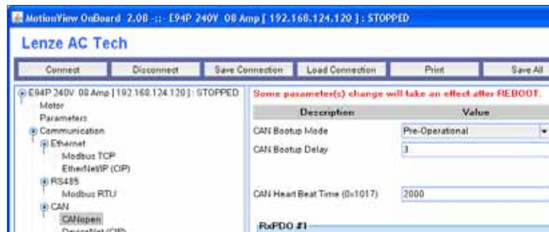
Figure 11: CAN Bootup Delay
