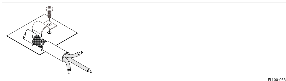
Fig. 6-3 CAN cable shield connection via cable clamp in the control cabinet
