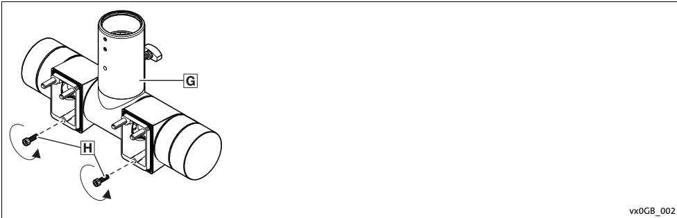
Fig. 2 Prepare the support arm adapter for mounting
