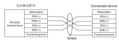
When connecting each of the signals with a twisted-pair cable, make the connections so that the RDA and RDB and the SDA and SDB become pairs of the twisted-pair cable. If the pair combinations are incorrect, a communication error may occur.
