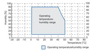
• Store the Panel PC within the ambient temperature and humidity ranges as shown in the following graph.
