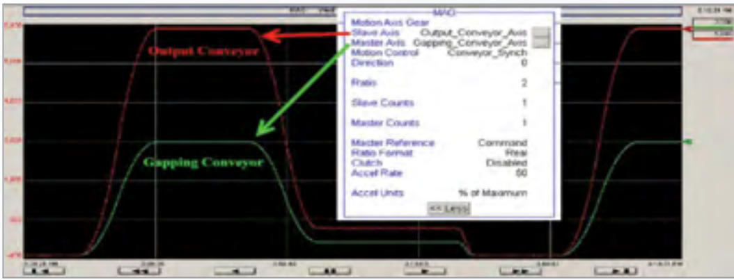
Easy-to-use motion instructions can synchronize two objects without the need for a large number of sensors, complicated mathematics or complex logic.
