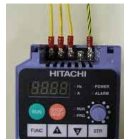
Input wiring for 3-phase input (models -NFU, -HFEF, -HFU)
