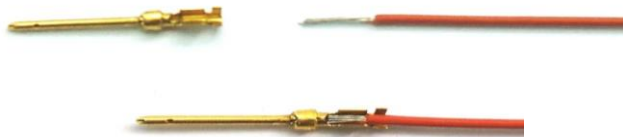
Figure 5-7 Making a communication cable
