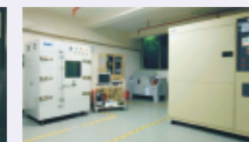
Faster temperature chamber & Thermal Shock Test Chamber
