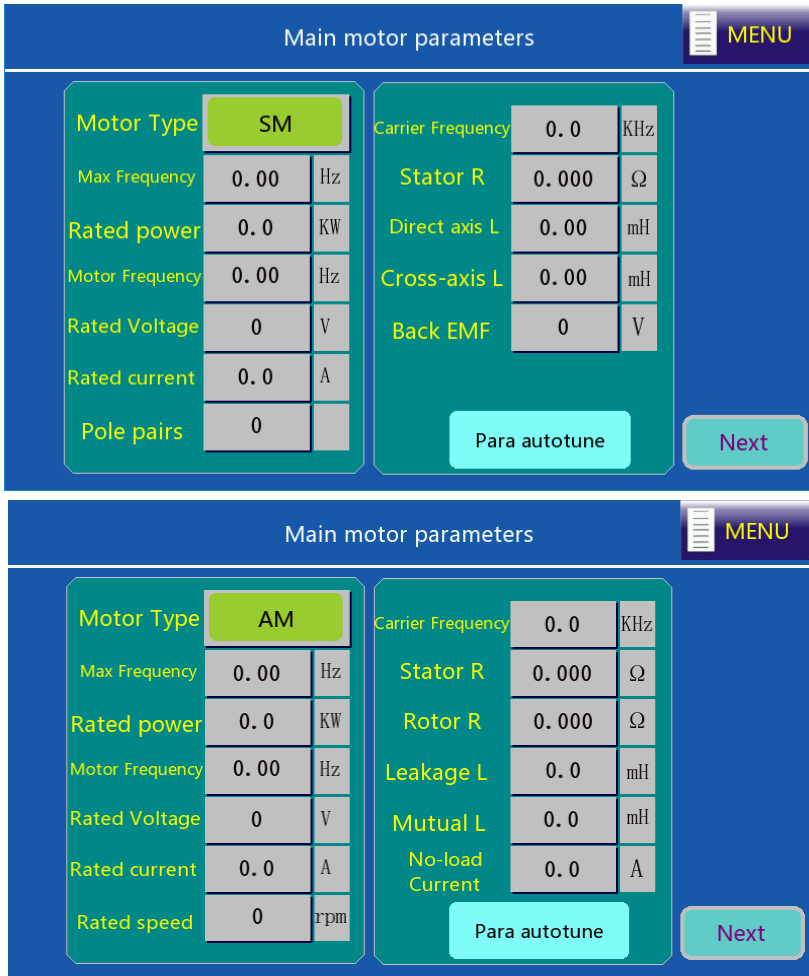
Figure 4-6 Main motor parameter setting interface
