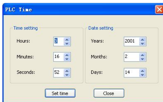
Figure 2-22 Setting PLC time
