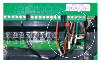
Optional PX-Brake Contactor Secure combines on one single board two options, the PX-Secure and the PX-Brake contactor, for more detailed information, refer to § 6.1.3 and 6.1.4.
