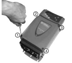
• Check that the DC bus voltage is below 40V before carrying out any work.
