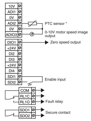
\* If the motor is not equipped with therminal sensor, ADI2 and 0V terminals must be strapped together.
