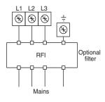
The customer connects the filter to the mains supply, without any special tools, on an IP66/Nema 4X dust and damp proof insulation displacement connector.
