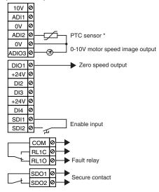
Operation : Run/Stop commands and the speed reference come from the optional keypad on PT or PB type drives. \* If the motor is not equipped with thermal sensor, ADI2 and 0V terminals must be strapped together.
