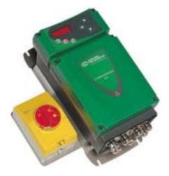
Optional PX-Disconnect is a lockable-IP66/Nema 4X tri-polar switch rated at 16A, with auxiliary contact NO-NF. PX-Disconnect is supplied fitted on a back plate ready to be mounted on the side of the drive.
