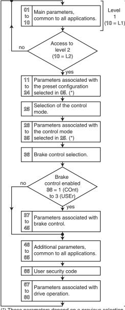
(\*) These parameters depend on a previous selection. As a result, they change from one configuration to the next. The number of parameters can also vary. In this case, the Commander SX will not offer unused parameters.
