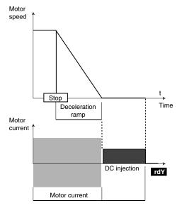
3 (dC-O) : stop by DC injection braking, and elimination at zero speed.
