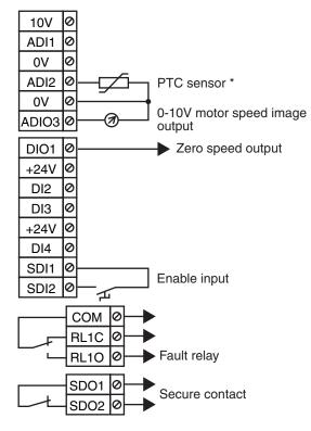
In this configuration, Run/Stop commands and the speed reference come from keypad.
