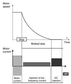
4 (dC-t) : stop on DC injection with an imposed period of time
