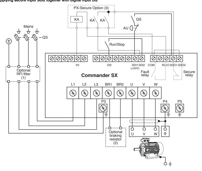
QS : Fused isolator : must be open before any maintenance intervention whether on motor - drive or any electrical components. AU : Emergency stop button
