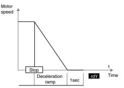
2 (rP.dC): stop on deceleration ramp with DC injection for an imposed period of time.
