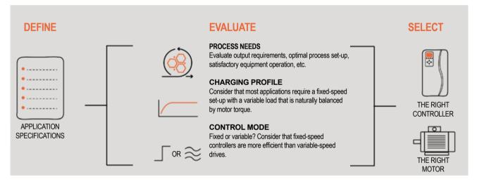
The Digistart starter range is optimised for use with IE3 motors. This is the most efficient control mode for a fixed speed and variable load system.
