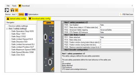
Besides the functionality shown in the picture it is possible to choose the STO either as hardwired input or via FSoE. Safe Brake Control is available as well.
