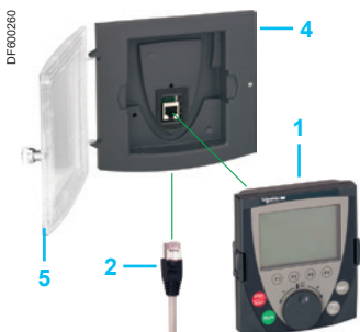
Using the remote graphic terminal on enclosure door: 1 + 2 + 4 (+ 5, if IP 65)
