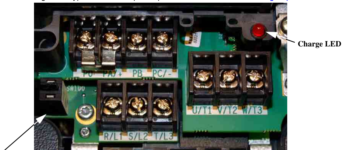
Figure 2. Typical G9 ASD Input/output Terminals and the Grounding Capacitor Switch .
