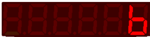
Figure 4.7: HMI screen when you select the option to perform backup of the control parameters to the flash memory card or vice versa
