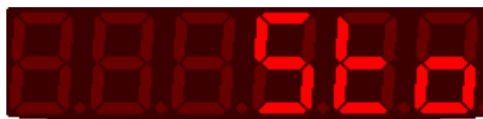
Figure 4.13: HMI screen when activating the safety function STO
