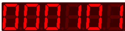
Figure 9.1: Example of status of DI1 to DI3
