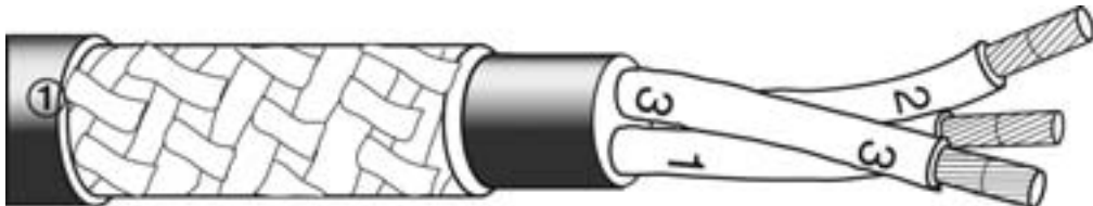
Galvanised steel or tinned copper wire with braided shield.
