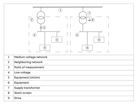
2. An EMC plan for preventing disturbances is drawn up for the installation. A template is available from the local ABB representative.
