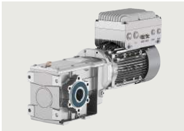
Example: Innomotics SG G115D distributed drive system, from our product partner Innomotics *), version with cable gland, FSA, 1.5 kW, motor LE 90, gearbox B49, hollow shaft
