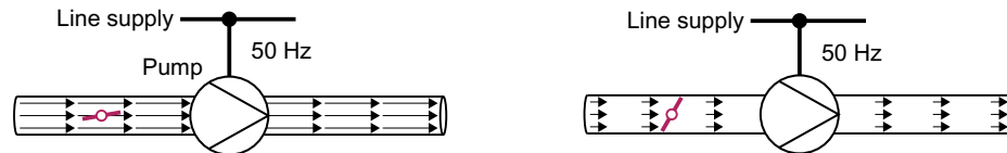
Figure 8-217 Flow control with pump and throttle connected to a 50 Hz line supply
