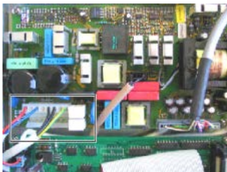
Switching power supply with connector on internal control voltage
