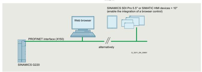
Integration of the SINAMICS web server based on the example of a SINAMICS G220 and the PROFINET interface (X150) as connected web client (e.g. PC, SIMATIC HMI etc.)
