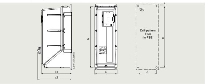
Principle dimension drawing and drill pattern for SINAMICS G220 degree of protection IP55 / UL Type 12
