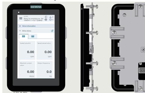
With the optional SINAMICS SDI Pro 5.5" door mounting kit, a SINAMICS SDI Pro 5.5" can be easily installed in a control cabinet door in just a few steps. The door mounting kit includes a metal plate for installing the SINAMICS SDI Pro 5.5" e.g. in a cabinet cutout. <sup>1)</sup> In case of door mounting with the SDI Pro 5.5" Operator Panel, the degree of protection IP55/UL type 12 enclosure is achieved for the front side.
