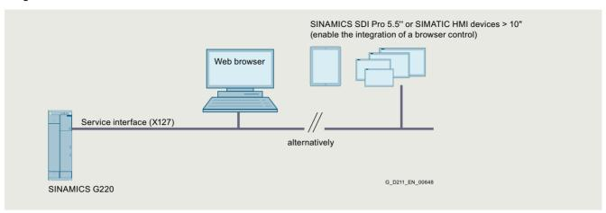
Integration of the SINAMICS web server based on the example of a SINAMICS G220 and the service interface (X127)
