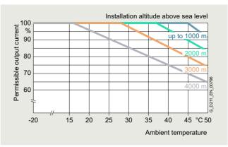
Permissible output current as a function of the installation altitude and the ambient temperature, SINAMICS G220 degree of protection IP55 / UL Type 12, at high overload (HO)
