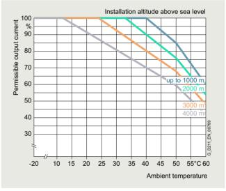
Permissible output current as a function of the installation altitude and the ambient temperature, SINAMICS G220 degree of protection IP20 / UL Open Type, at operation with synchronous reluctance motor
