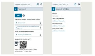
The additional available options in the form of the SINAMICS SDI Pro 5.5" handheld kit and SINAMICS SDI Pro 5.5" door mounting kit extend the operating range of the device. With the SDI Pro 5.5" handheld kit, the device can be equipped with a rubber oversheath for mobile use. The SINAMICS SDI Pro 5.5" door mounting kit enables the SINAMICS SDI Pro to be installed in control cabinet doors.
