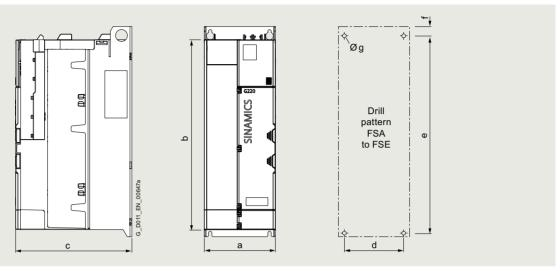
Principle dimension drawing and drill pattern for SINAMICS G220 degree of protection IP20 / UL Open Type
