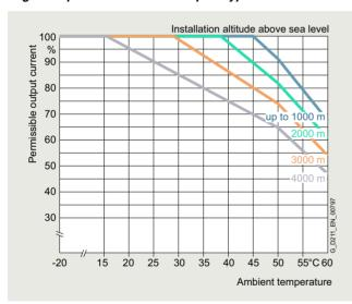
Permissible output current as a function of the installation altitude and the ambient temperature, SINAMICS G220 degree of protection IP20 / UL Open Type, at low overload (LO)
