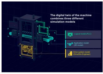
DriveSim Engineer is an innovative solution that combines drive simulation and virtual commissioning. With this powerful combination, you can optimize your drive systems, test and validate your projects and ensure that your drive systems function correctly prior to the installation.
