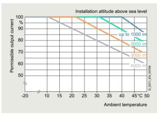
Permissible output current as a function of the installation altitude and the ambient temperature, SINAMICS G220 degree of protection IP55 / UL Type 12, at low overload (LO)
