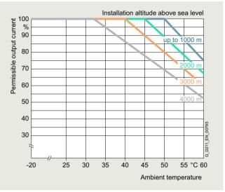
Permissible output current as a function of the installation altitude and the ambient temperature, SINAMICS G220 degree of protection IP20 / UL Open Type, at high overload (HO)
