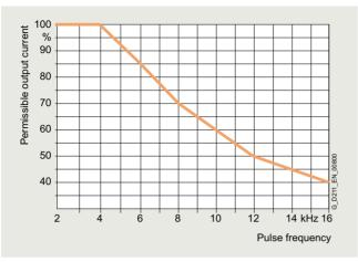
Permissible output current as a function of the pulse frequency, SINAMICS G220, at low overload (LO)
