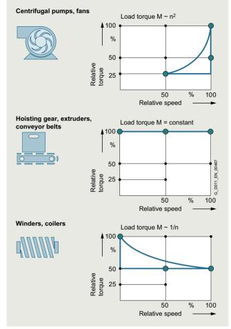
Duty cycles for different driven machines
