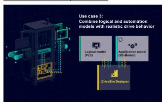
With the third Use case, you can connect a simulation tool such as NX Mechatronic Concept Designer to visualize the mechanical movements of your application. This way, you ensure that the drive behaves according to the desired machine performance. You can test several fault scenarios and optimize the interaction between PLC, application and drive virtually so overall, you can avoid unplanned machine behavior and increase the performance of your setup.
