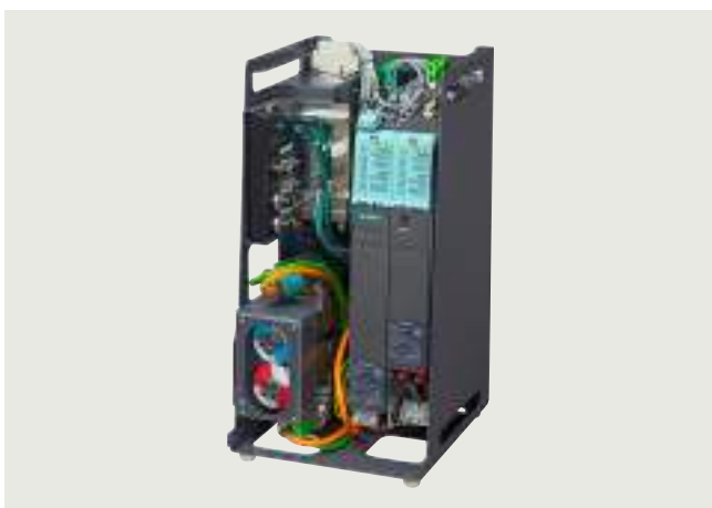
SINAMICS S120 training case without Control Unit
