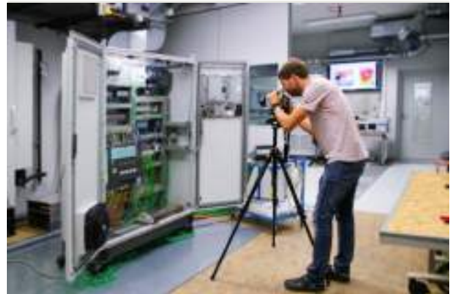
WKC - Test laboratory - Heat measurement
