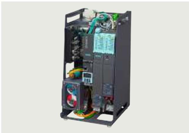
SINAMICS S120 training case with CU320 Control Unit
