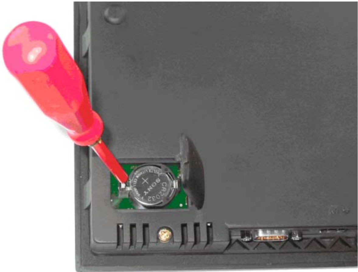
Figure 11-22 Replacing the backup battery for the cabinet operator panel
