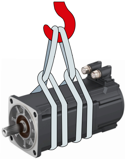
Figure 5-2 Lifting and transporting with lifting slings (example diagram)
