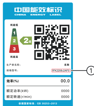
Figure A-1 ① Article number (diagram showing a typical 1FK2, is also applicable for 1FT2)
