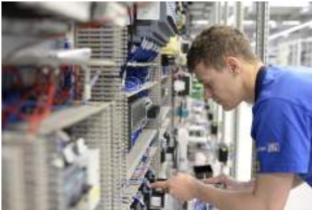
WKC - Control cabinet wiring
