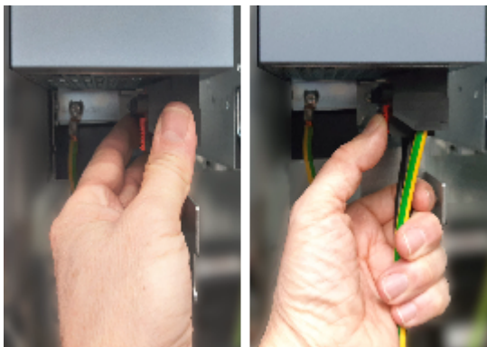
Figure 7-22 Releasing the power connector
